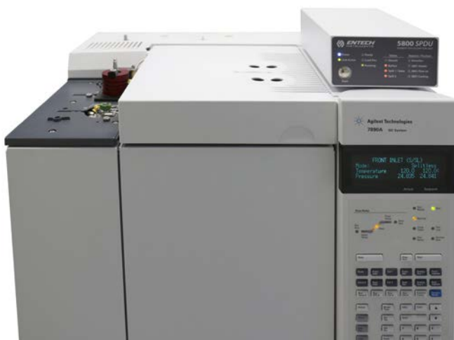
Figure 7 - 5800 SPDU shown on Agilent GC. After sample extraction, simply insert the Sorbent Pen into the 5800 SPDU and press START on the 5800 Controller to transfer volatile to semi-volatile compounds onto the column and to the detector for sensitive and accurate analysis.
