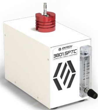
Figure 4 - To prepare new Sorbent Pens for extraction, the 3801 Sorbent Pen Thermal Conditioner (SPTC) is used to condition Sorbent Pens prior to use up to 350°C depending on the sorbent type. During the analysis, the Sorbent Pens are both desorbed to the GCMS and thoroughly baked out, eliminating the need for additional thermal conditioning before reuse. However, if a Sorbent Pen was not isolated after extraction or if it contained unusually high concentrations of extracted compounds not completely removed during the previous analysis, the 3801 SPTC can be used for a quick cleanup of the Pen.
