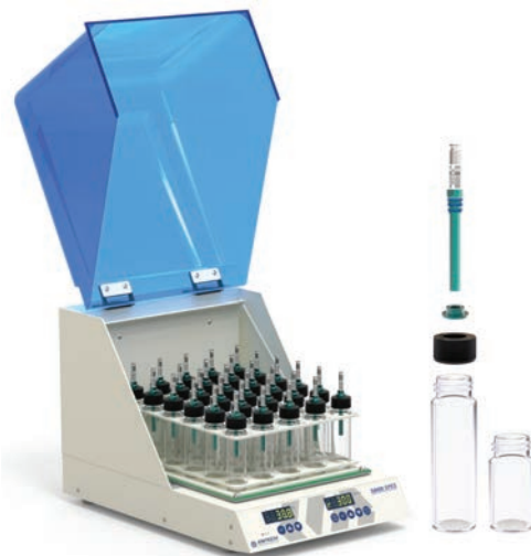
Figure 5 - Sample vials and agitator used to perform VASE. The 5600 Sorbent Pen Extraction System (SPES) provides a convenient way to perform vial extractions using 30-position trays, allowing for significant sample throughput. The sample to be extracted is loaded into the vial, the Sorbent Pen is inserted, a vacuum is created through the MicroQT seal at the top of the Pen, and the sample is loaded onto the tray. The extraction time, temperature, and RPM can be programmed on the 5600 SPES and the vacuum extraction process begins. The Sorbent Pen Extraction System agitates the samples at 30-300 RPM to speed up transfer of volatiles to the headspace, while controlling the sample temperature from 4°C to 70°C. Extractions can be completed in 1–48 hours depending on the application.
