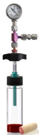
Figure 1 - The vacuum tight seal allows samples to remain under vacuum after a 30 second evacuation, which allows elevated rates of static diffusion to collect significantly more headspace compounds on the adsorbent than can be collected at atmospheric pressure. Sorbent Pens are labeled with a bar code sticker to allow the operator or autosampler to simply scan the Sorbent Pen into the sequence table. The bar code also allows the tracking of each Sorbent Pen through its lifetime of hundreds to thousands of extractions and desorptions.
